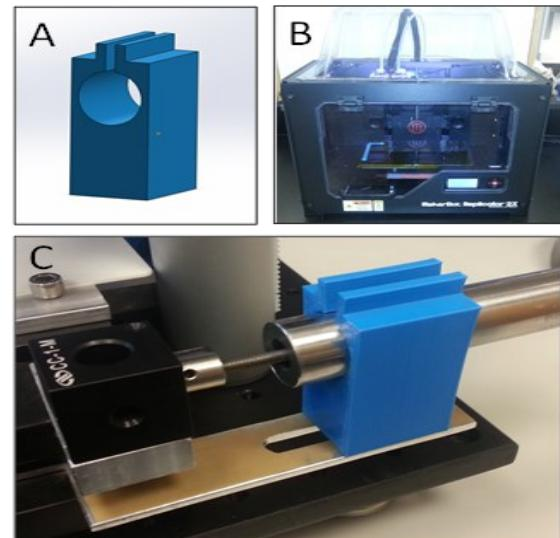
**Figure 1:** Development in CAD (A), manufacture (B), and use (C) of part that requires precise alignment and tolerancing that was manufactured with the 3-D printer.
