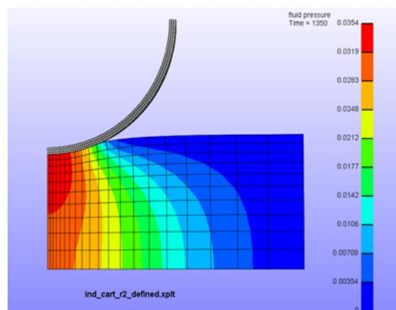
**Figure 2:** FE Model of biphasic cartilage indentation.
